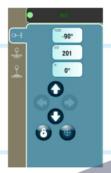
Tube stand movement controls on the main imaging console screen, allows position fine-tuning from the operator room.
